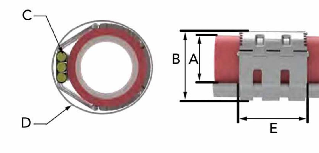
A Tubing O.D. C Cable Size E Protector Length B Collar O.D. D Runing O.D.
