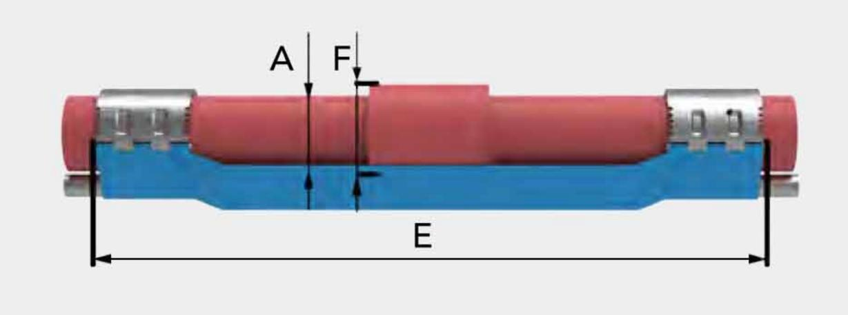
A Tubing O.D.B Collar O.D.E Protector LengthC Cable SizeF Coupling O.D.
