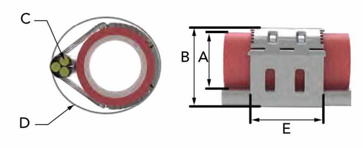
A Tubing O.D. C Cable Size E Protector Length B Collar O.D. D Runing O.D.
